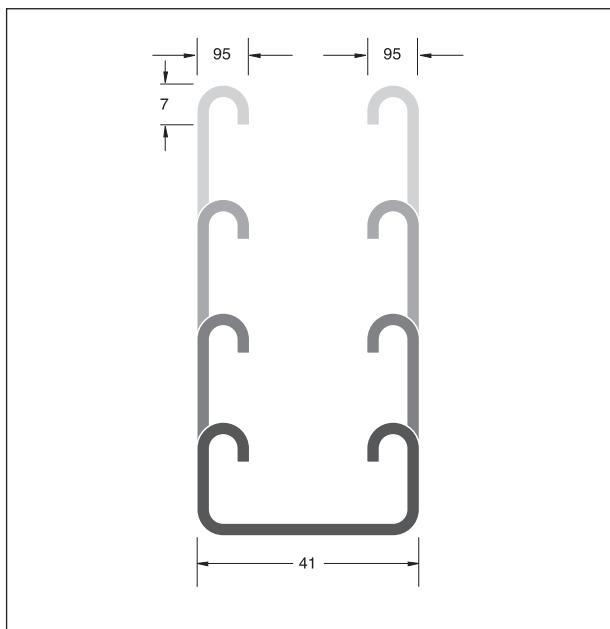
Standard Kwikstrut channel ensures a high load carrying capacity whilst the thinner Uni range channel provides economical support for lighter loads, maintaining total flexibility in the design and construction of assemblies required for framing applications.
