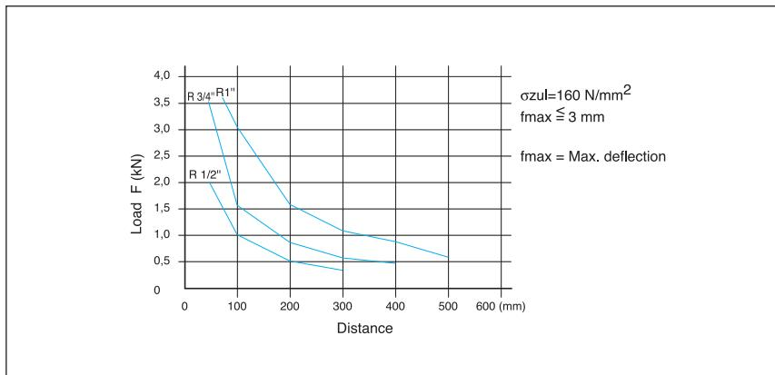
Note: The loads are only an example for an anchor bolt type FAZ in cracked concrete C20/25 resp. B25. When using other anchors or anchor bolts or other fastening grounds the load has to be calculated accordingly.
