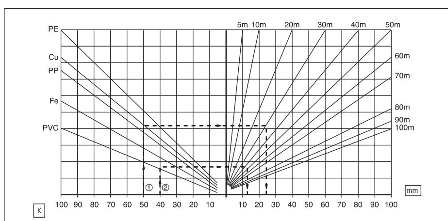
Note: Plastic pipes (PE, PP, PVC) multiply the expansion value from the chart by 10.
