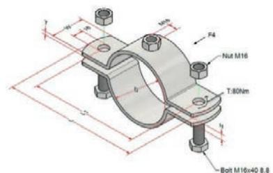
In the example above the non-insulated fix point is used in combination with fix point bracket FPBRACK17
